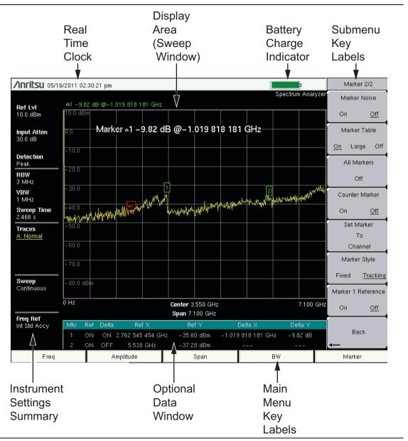
Figure 2-6. Spectrum Analyzer Display
