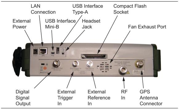
Figure 2-12. Test Panel Connectors for MS8911B
