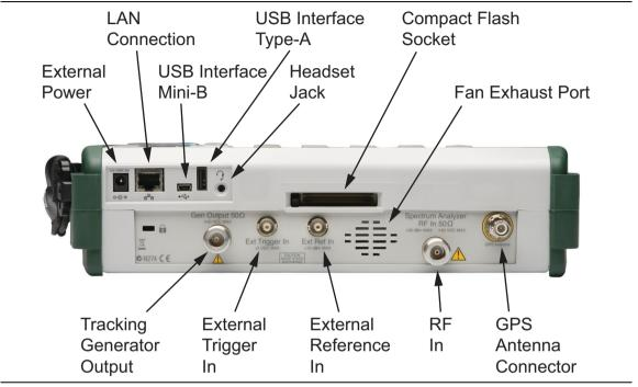
Figure 2-10. Test Panel Connectors for MS2721B
