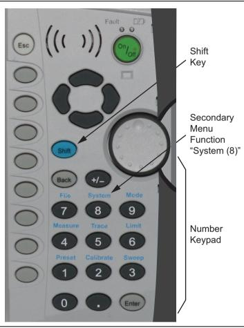
Figure 2-5. Keypad and Secondary Function Menus
