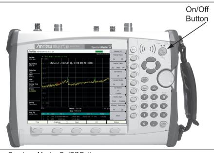
Figure 2-1. Spectrum Master On/Off Button
