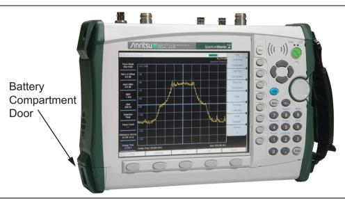
Figure 1-1. Battery Compartment Door
