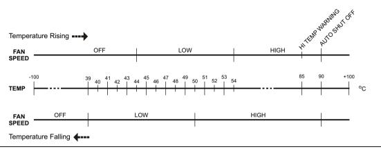
Figure B-1. Fan Speed versus Temperature
