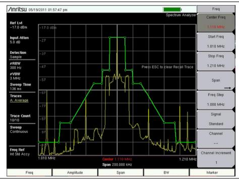
Figure 3-2. Complex Limit Line Example
