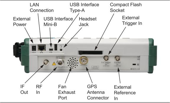
Figure 2-11. Test Panel Connectors for MS2723B and MS2724B
